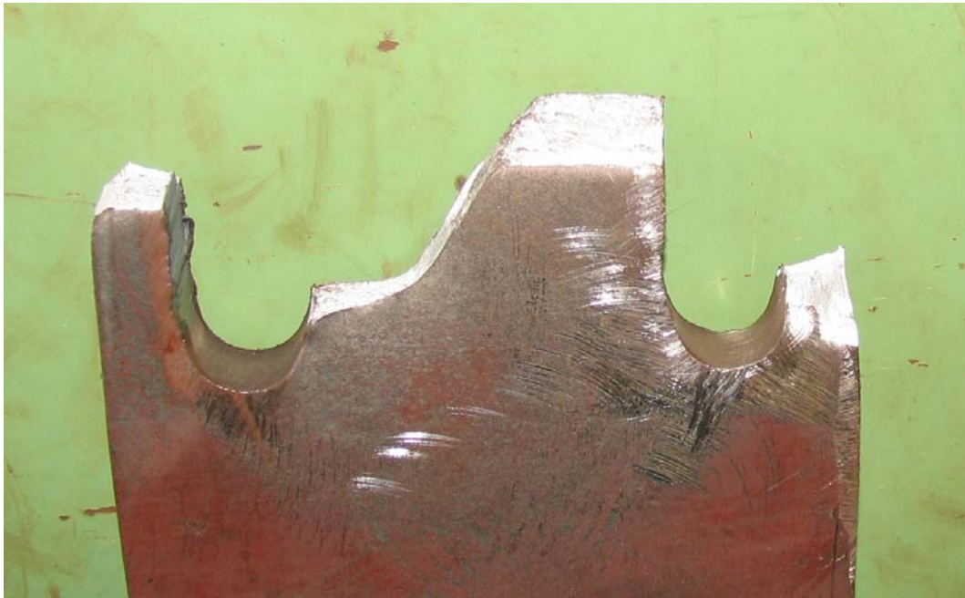
Figure C-29 Failure of drilled plasma Grade 50 3/4" specimen
