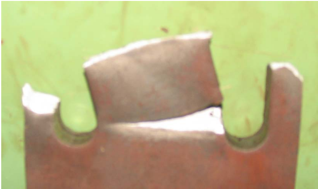
Figure C-26 Failure of punched full size Grade 50 \frac{3}{4} \"specimen
