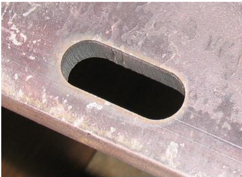
Figure 1-6 – Slotted laser cut hole
