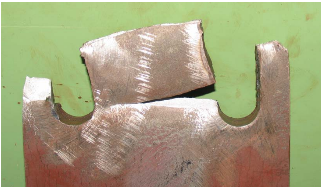
Figure C-30 Failure of punched plasma Grade 50 3/4" specimen
