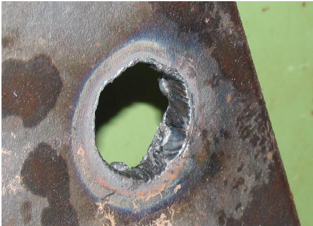
Figure 1-4 Typical oxy act hole
