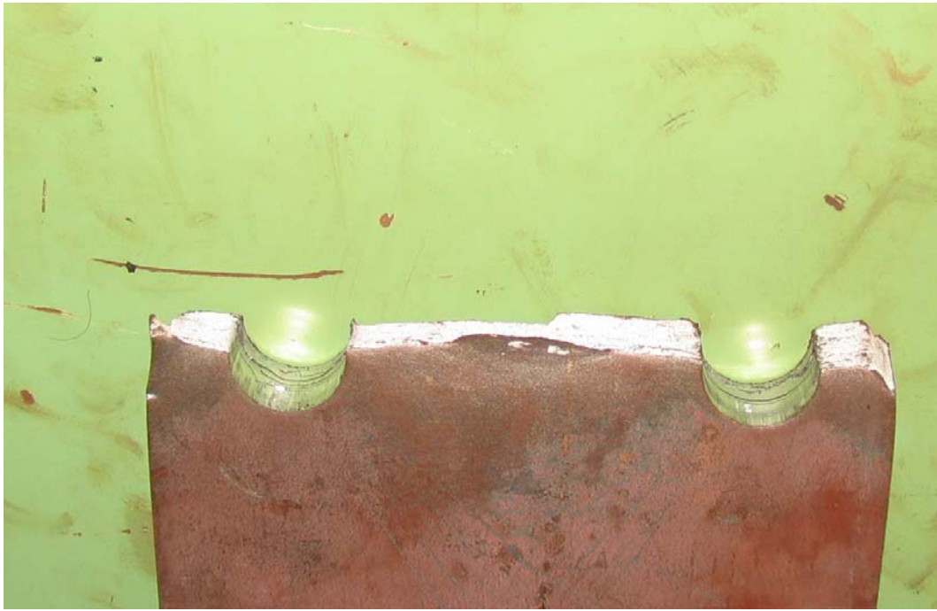
Figure C-25 Failure of punched round hole Grade 50 \frac{3}{4} \"specimen
