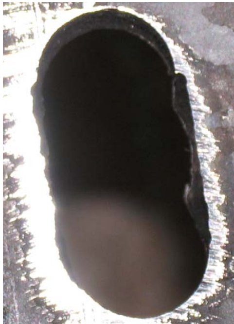
Figure 4-10 Typical plasma cut hole
