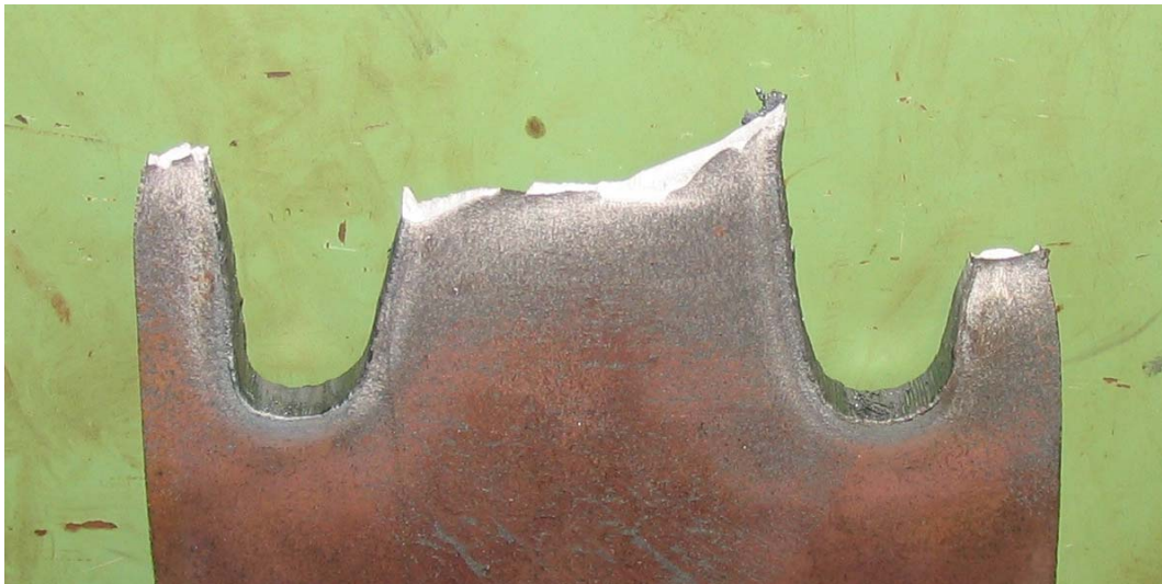
Figure C-12 Failure of oxy act full size Grade 50 3/8" specimen
