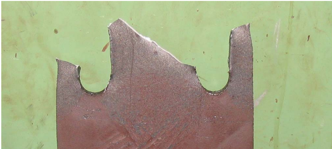
Figure C-20 Failure of drilled plasma Grade 50 3/8"specimen
