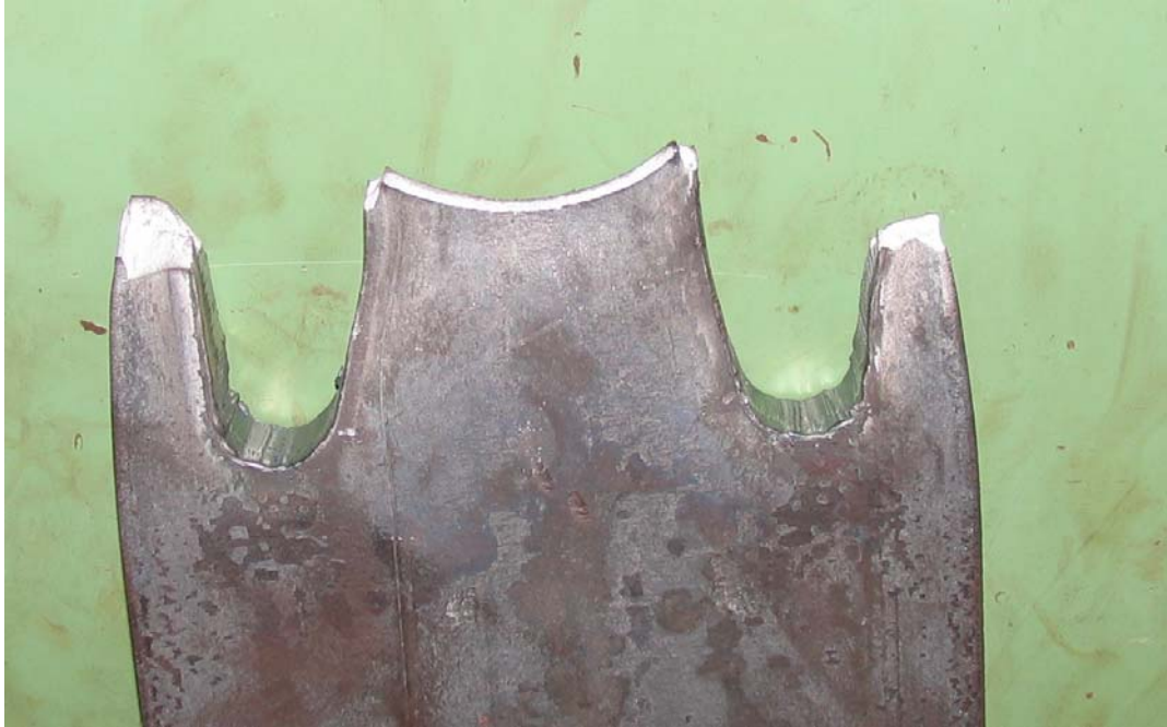
Figure C-1 Failure of Oxy act full size A36 3/4" specimen
