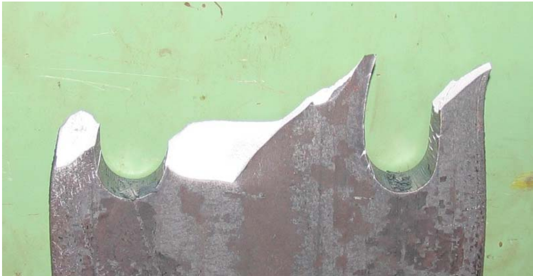
Figure C-7 Failure of laser cut hole A36 3/4"specimen
