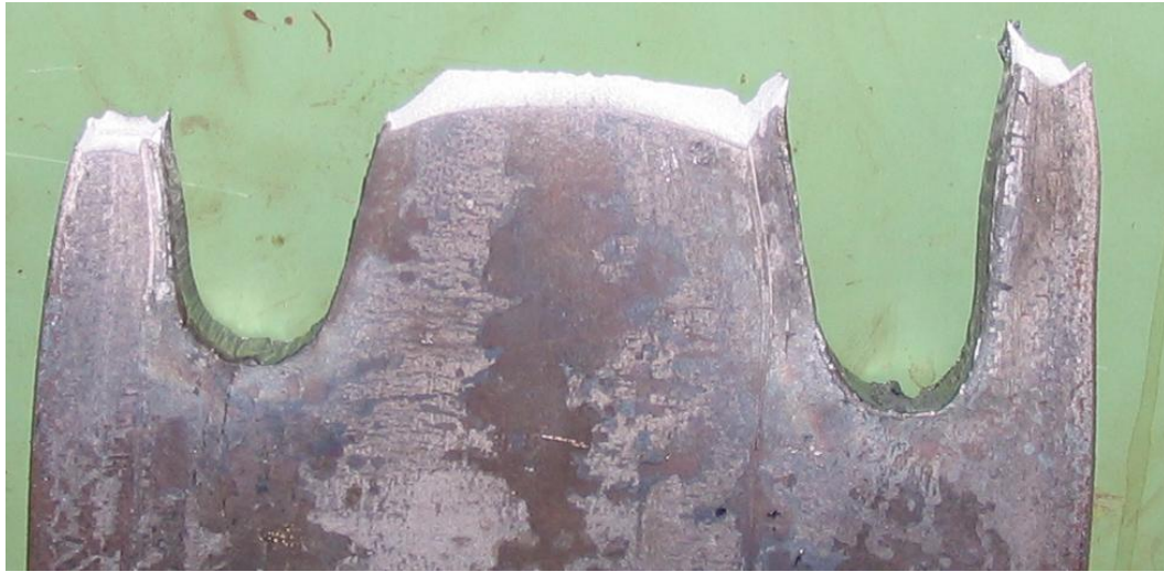
Figure 5-7 Single plane failure of A36 steel specimen
