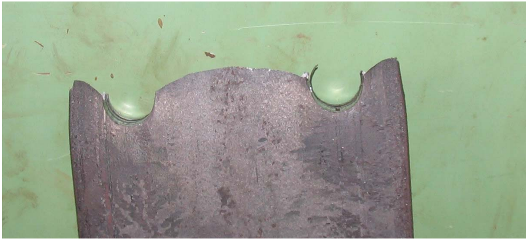
Figure C-5 Failure of punched round A36 \frac{3}{4} \"specimen
