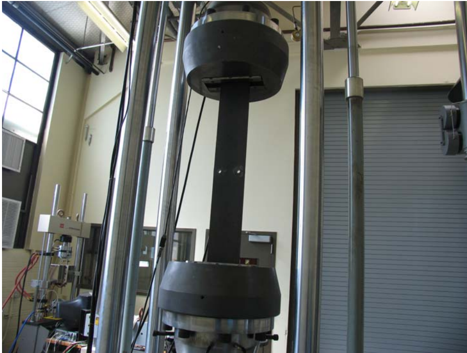
Figure 4-13 Cyclic tests set up
