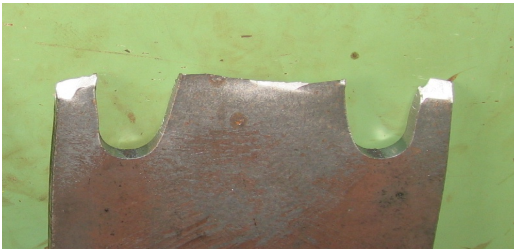
Figure C-18 Failure of Laser cut full size Grade 50 3/8"specimen
