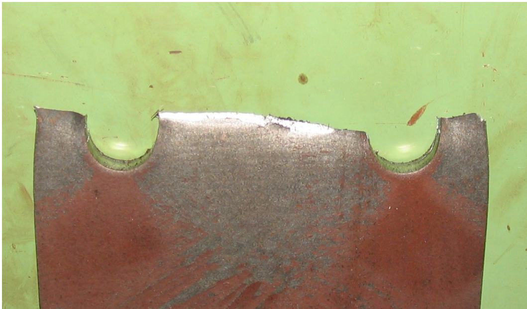
Figure C-16 Failure of punched round hole grade 50 3/8"specimen
