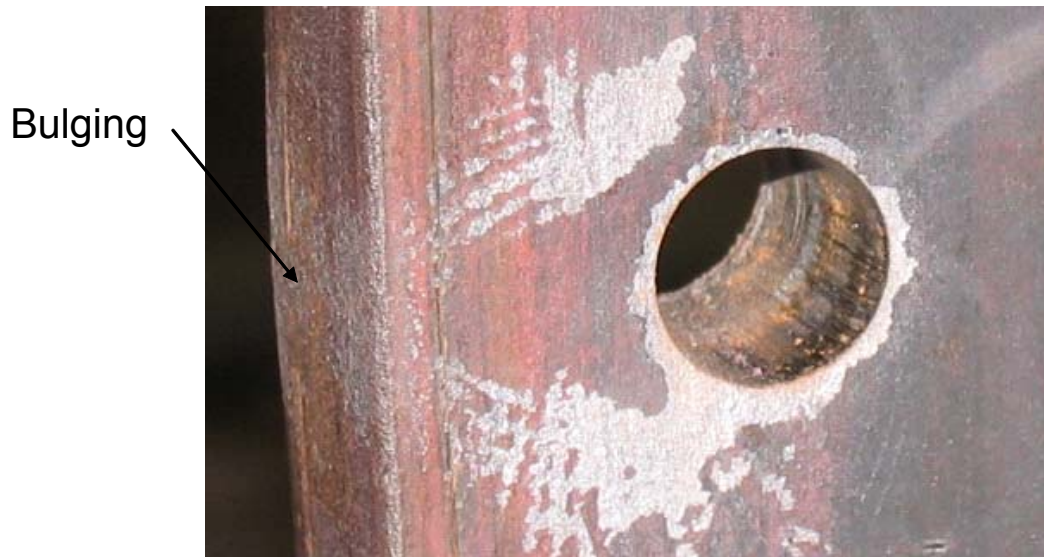
Figure 5-14 Example of bulging created hole punching
