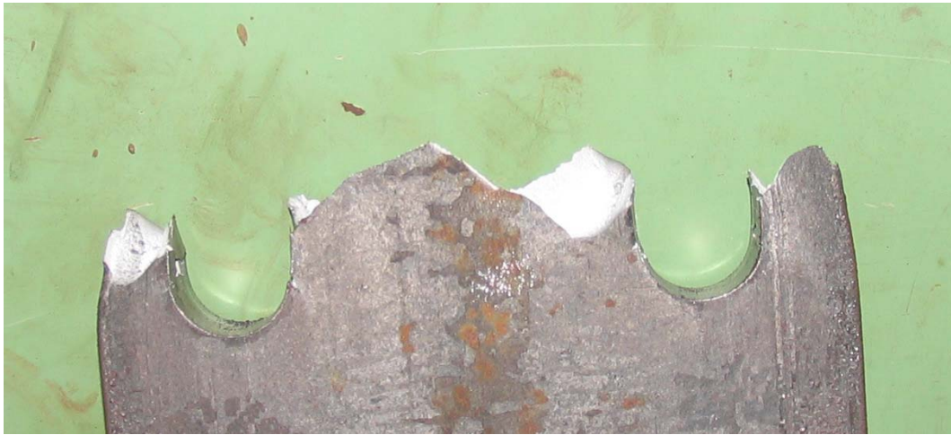
Figure C-11 Failure of short slotted A36 3/4" specimen
