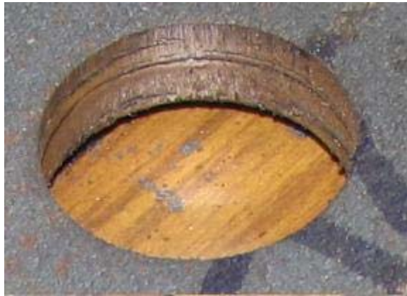
Figure 3-10 Punch hole made in 3/8" plate with 1/32" die clearance
