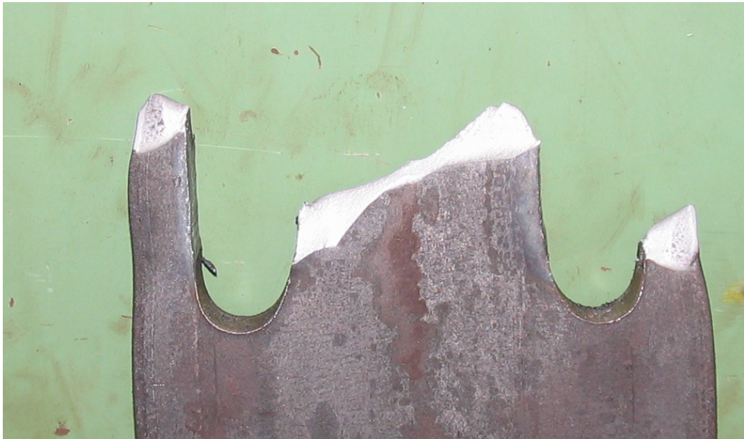
Figure C-9 Failure of drilled plasma A36 3/4" specimen
