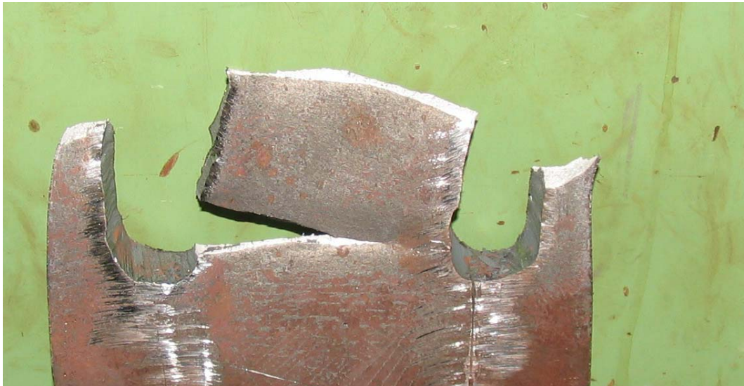
Figure C-28 Failure of Plasma cut full size Grade 50 3/4"specimen
