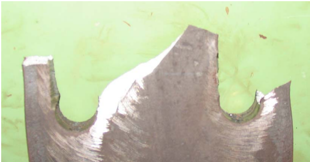
Figure C-10 Failure of punched plasma A36 3/4" specimen
