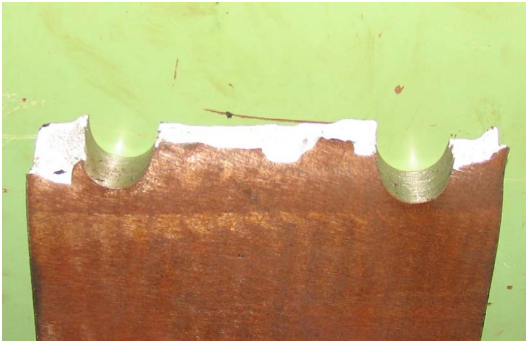
Figure C-24 Failure of drilled round hole Grade 50 \frac{3}{4} " specimen
