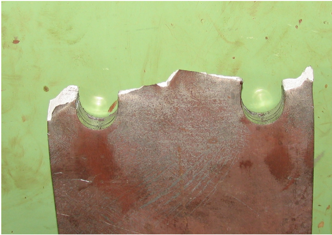
Figure C- 31 Failure of short slotted holes Grade 50 \frac{3}{4} "specimen
