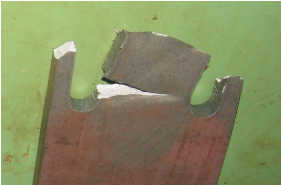
Figure C-27 Failure of laser cut full size Grade 50 3/4"specimen
