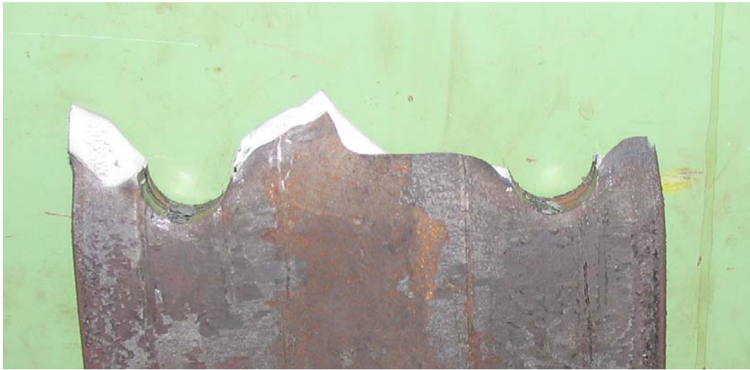
Figure C-3 Failure of punched – oxy A36 3/4" specimen
