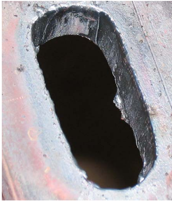
Figure 4-9 Typical full size oxy acetylene slotted hole
