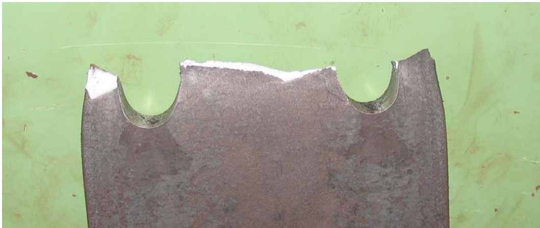
Figure C- 4 Failure of drilled round A36 3/4"specimen
