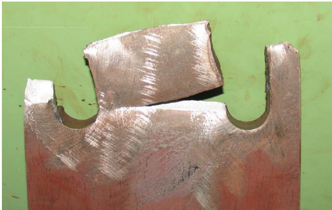
Figure 5-8 Brittle fracture of punched plasma Grade 50 \frac{3}{4} " plate
