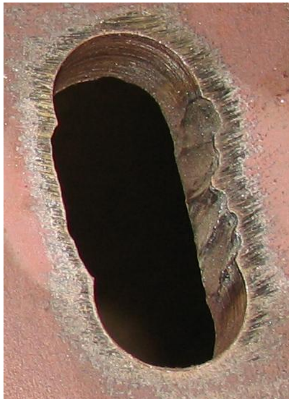
Figure 1-9- Punched holes joined with oxy-act cut
