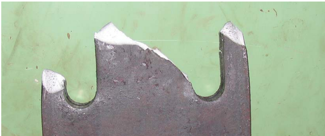
Figure C-6 Failure of Punched full size Long slotted hole A36 \frac{3}{4} \"specimen
