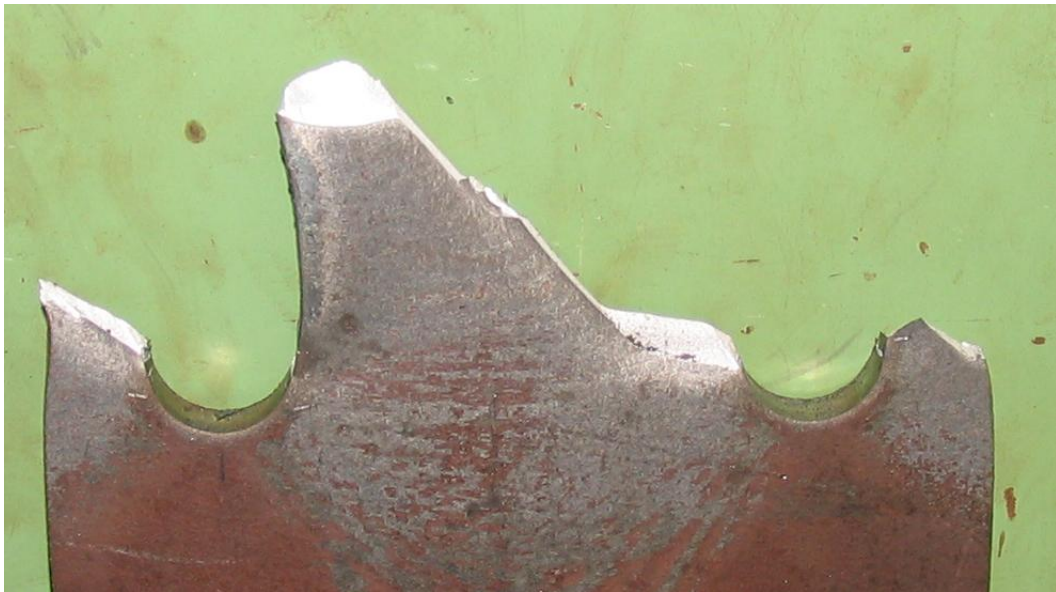
Figure 5-5 Typical failure for Grade 50 steel 3/8" plate
