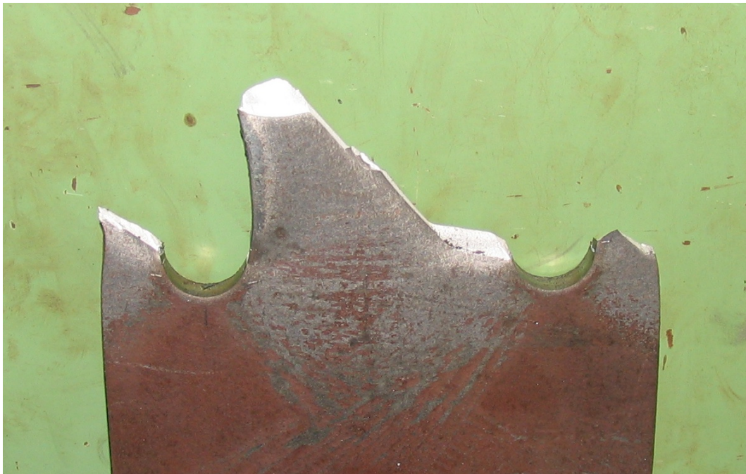
Figure C-14 Failure of punched oxy Grade 50 3/8"specimen
