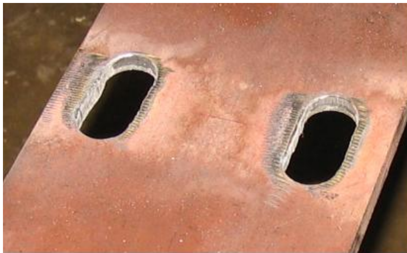
Figure 4-2 Phase 2 of making of slotted holes
