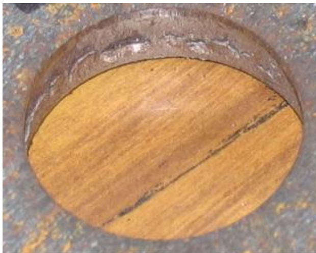
Figure 3-11 Punch hole made in 3/8" plate with 1/16" die clearance
