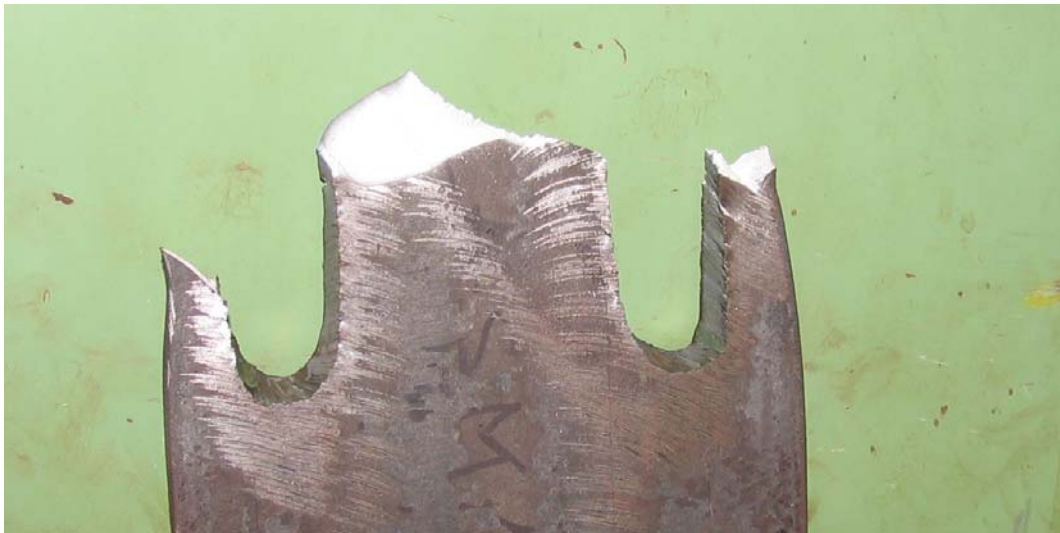
Figure C-8 Failure of Plasma cut full size A36 3/4"specimen
